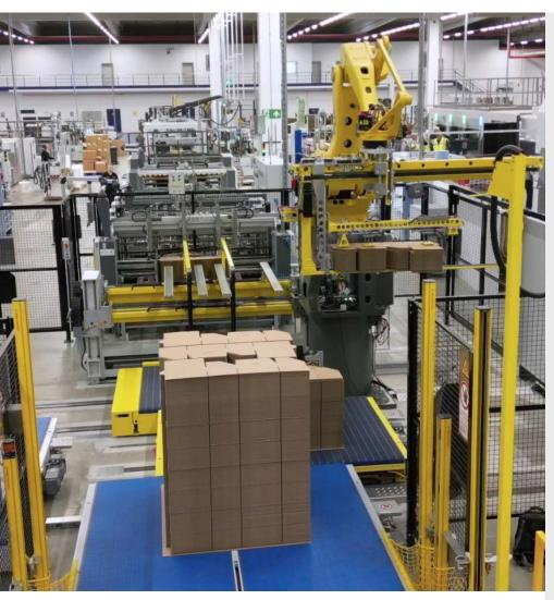
POWERPACKER in its 4th generation with well known, global strapping system suppliers equipped, grants a perfect bundle which is transferred to our palletizing robot system.
