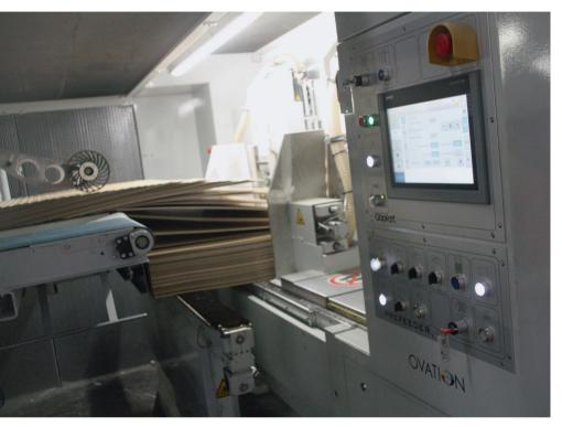
can feed several die-cutters. The Göpfert pre-feeder and vacuum lead edge feeder uses belts instead of friction rolls in order to eliminate marks on the liner when using coated papers and running E and F-flute sheets. The optional sheet cleaner removes dust from the sheet prior printing. The high end inking system with chamber doctor blade system and ceramic anilox roll system ensures excellent print quality. The tool-less doctor blade clamping system makes maintenance easy for the operators.
