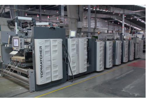
The machine is able to handle multi-piece boxes of almost any kind from 140mm in width and 140mm feed length for the upper part of the box and 455mm in width and as low as 160mm in feed length for
