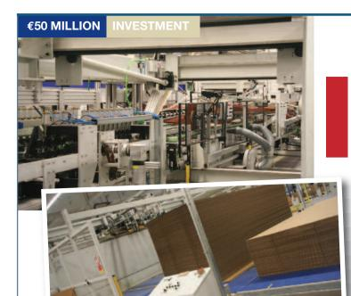
running register adjustment and an extended slotting capability. When used in combination with the rotary die-cut unit, the Container Line is capable of producing product in a wide range of shapes and sizes.
